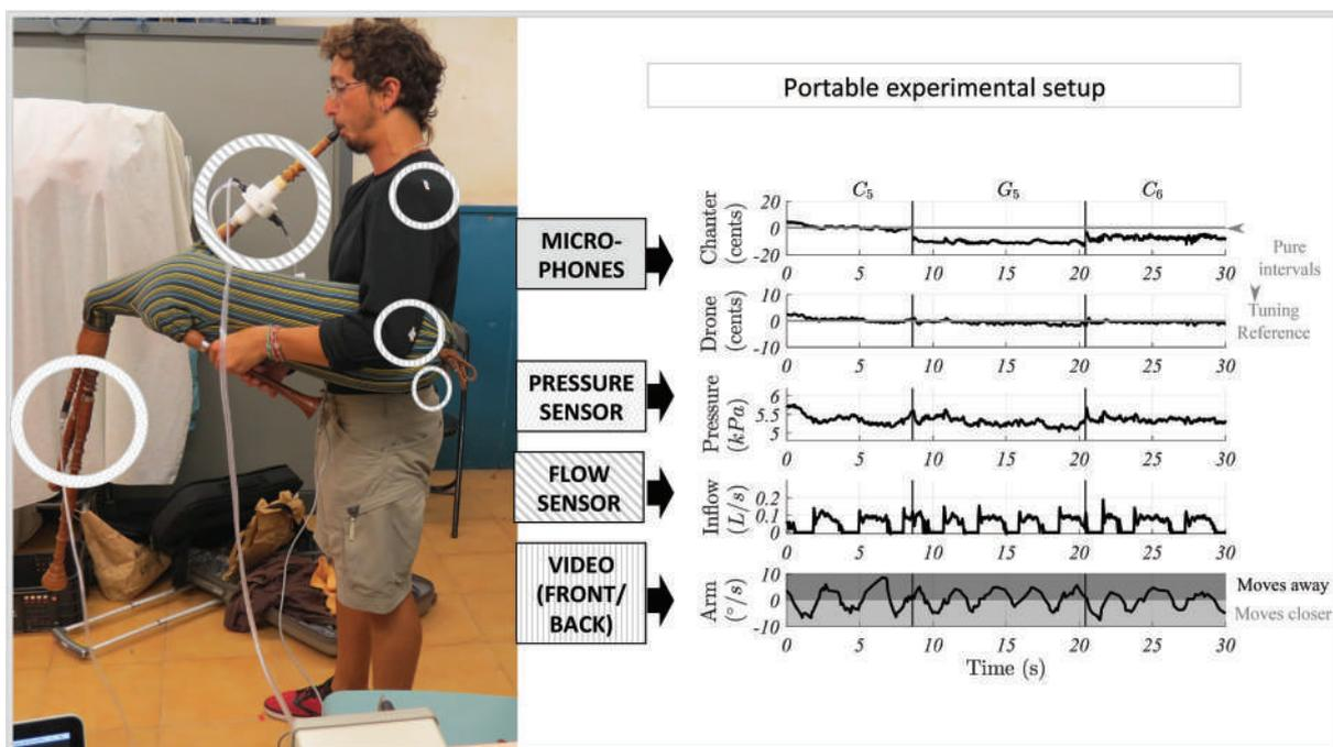
Figure 2. Portable experimental set-up on Mallorcan xeremies with an example of the results.
