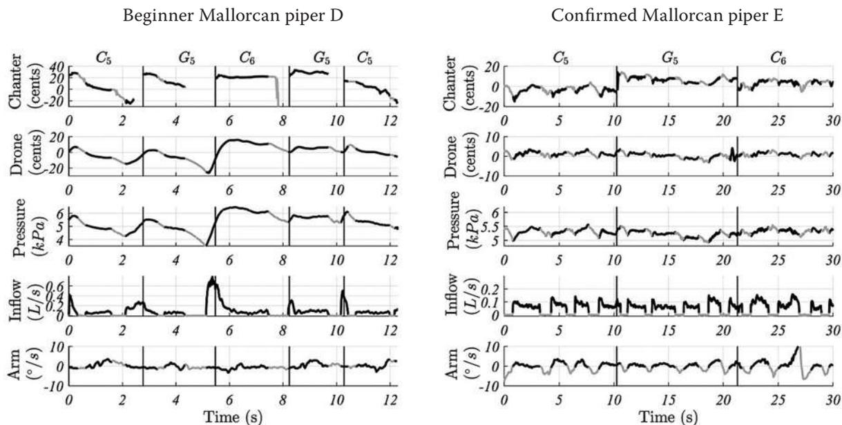
Figure 4. Proficiency comparison between a beginner (D) and a confirmed xeremies player (E) performing an arpeggio exercise (C5, G5, C6). The black sections indicate when the arm is moving away from the body; the grey sections indicate when the arm is towards the body. Each vertical line indicates a different note. Note: the pitch, pressure and inflow scales are different for both pipers. The scale for piper 'E' is much smaller than for piper 'D'. Source: Ernoult et al. (2017), p.1460.
